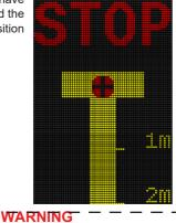
Stop the aircraft if the display shows: STOP Wrong aircraft type/series Led display is deactivated.
